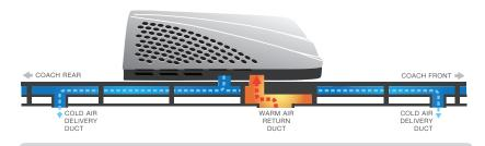
How it works: The Quiet Zone System feeds cool air directly into the ductwork system. Cool air enters a port built into the rafters at the first stage of distribution. Warm air is pulled through a separate ductwork system to be vented to the outside. This residential style system keeps noise and vibration away from the living space for quiet, cool comfort.
