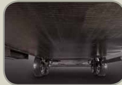
Heated and enclosed underbelly protects your coach and improved airflow allows for a sturdier ride.
