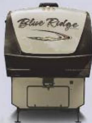
The two-color aerodynamic front end has LED lights for easy hitch hook-up.
