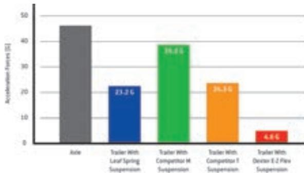
Compare acceleration forces experienced by an axle and trailer while traveling over railroad tracks at 30 MPH. The E-Z Flex® System provides up to an 80% reduction in forces on the trailer frame vs. a standard equalizer. E-Z Flex® significantly outperforms all other competitors in the same road test for a smoother, more protective ride for your trailer and cargo.
