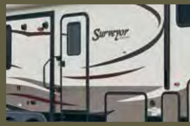
SIDEWALL 2-TONE GEL-COATED FIBERGLASS SIDE WALLS WITH PREMIUM GRAPHICS
