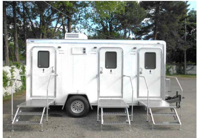
Side View showing Steps, Railings, & Porches Assembled
