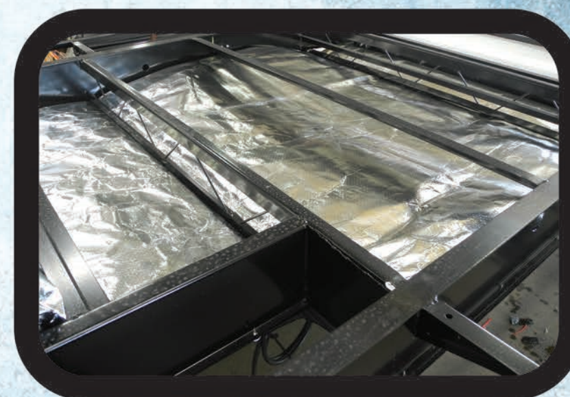
Radiant Foil Insulation on Roof, Floor, Slideout Floor and Nose
