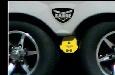
Upgraded EQUA FLEX suspension increases vertical travel for smooth towing
