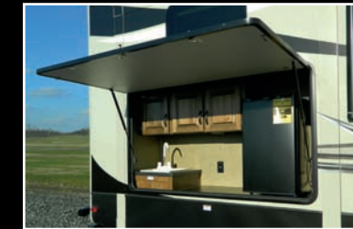
Outside kitchen is equipped with refrigerator and sink in slam-latch compartment
