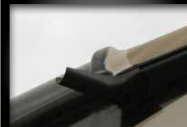
Drip rail with extra long drip spouts help prevent black streaking.
