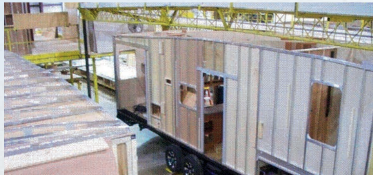
Aluminum studded sidewalls and roof trusses on 16" centers or less
