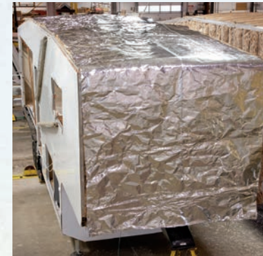
R-38 Radiant shield Thermo-foil wrap through ceilings, underbellies and under front cap.
