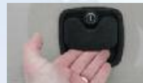
Slam-Latch baggage doors are on all exterior compartment doors, except the LP tank door.
