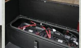
**ENCLOSED BATTERIES** Two batteries in a single housing for easy access.
