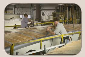
A full length 3/8" wood decking, for a full walkon roof, is screwed, not stapled, into place. Our final step is adding a twoply, Tuff ply™, rubber roof membrane with a built-in fire retardant and 12 year warranty.
