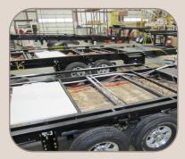
Black, Grey, and Fresh Water tanks are installed with individual 12-volt, large surface heating pads on *ALL* tanks. These tank heaters allow for all season camping. Competitors install a one piece underbelly design which is screwed into the frame.
