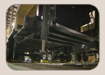
jacks are tested right on the production line to ensure proper working order. This process eliminates air bubbles within the hydraulic
