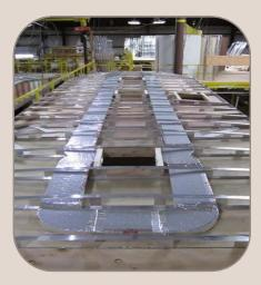
Our 5" aluminum roof rafters allow us to run a full 8" wide, race track, duct system. This allows more ducted air flow compared to our competitors 5" wide duct. Circular ducting ensures uniform cooling with (1) standard air conditioner or upgrading to an optional 2 air conditioning system.
