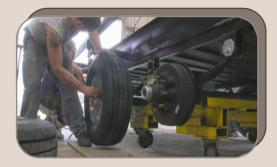
Heavy Duty, E-Z<sup>™</sup> Lube, Dexter Axles with ST "E" & "G" Rated Tires (#6000 and #7000 axles) Makes bearing lubrication quick and easy, with no disassembly required.
