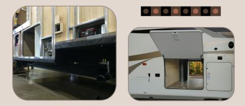
The purpose of the tripod is to build every unit like it's hooked to your vehicle as it is traveling down the road. Common practice in the industry is to put roller wheels on the front jack legs, but not at Cedar Creek. The flex of a frame is different when it is sitting on the truck. This practice ensures a level coach, each and every time, and creates a tighter fit and finished frame.
