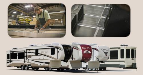
**Purchased Laminated Sidewalls** are the most commonly produced sidewall in the industry. These walls start with a welded frame that generally runs every 24-"48" on center. Welded frames are not designed for strength, but for parameter structure. Polystyrene foam is placed inside the framework. The interior wall board and exterior materials are either
