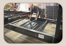
Inserted into each Steel frame is our one of a kind, ABS, impact resistant, waterproof, underbelly. Each 4' x 8' ABS panel is inserted front to back, inside each frame. The panels are then anchored into a braced wood backer within the frame.
