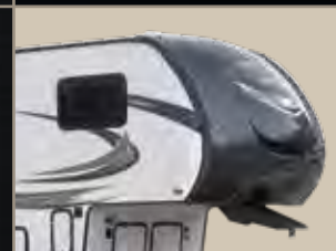
Painted gel coat fiberglass front cap with light strips on Fifth Wheels, won't fade, chalk or crack
