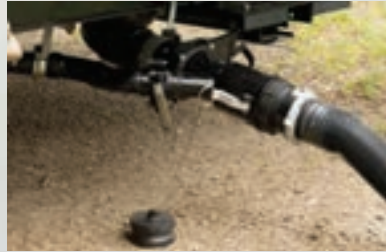
WASTE MASTER SEWAGE MANAGEMENT SYSTEM Rugged for quick, easy and sanitary waste disposal. (N/A LE, MBS and Transit)
