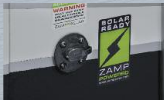
SOLAR PREP Easily charges the 12V system with aftermarket solar panels.
