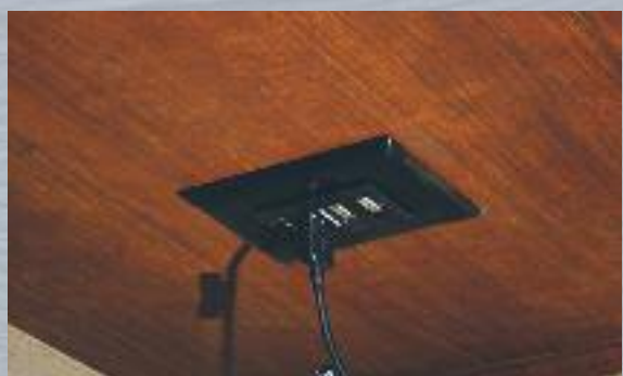
USB CHARGING STATION 12V 4-port USB charging station (Living room/bedroom)
