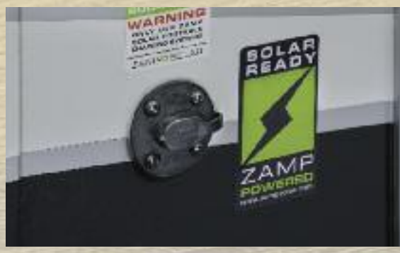
SOLAR PREP Easily charges the 12V system with aftermarket solar panels.
