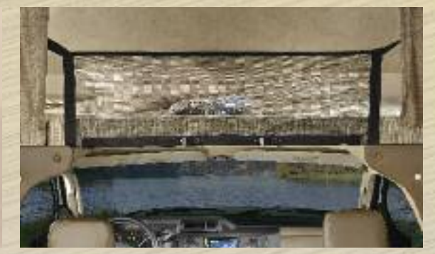
CAB OVER BUNK SAFETY NET The overhead bunk is rated for 440 lbs.
