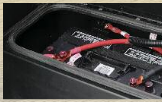
ENCLOSED BATTERY One battery in a single housing for easy access.
