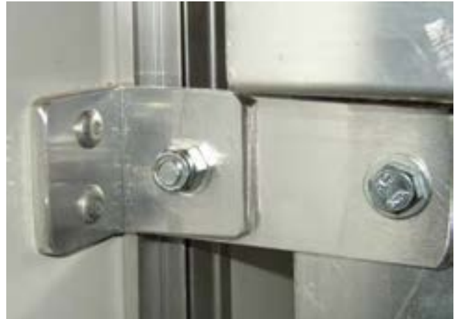
Bracket - Holds Porch in Retracted Position
