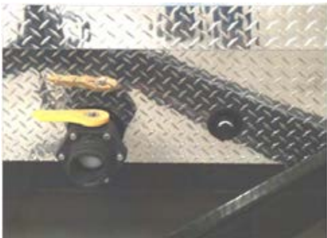
Front of Trailer Showing Pump Out Valve and Wash Out Port
