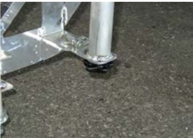
View of Rail Locking Pin at Bottom
