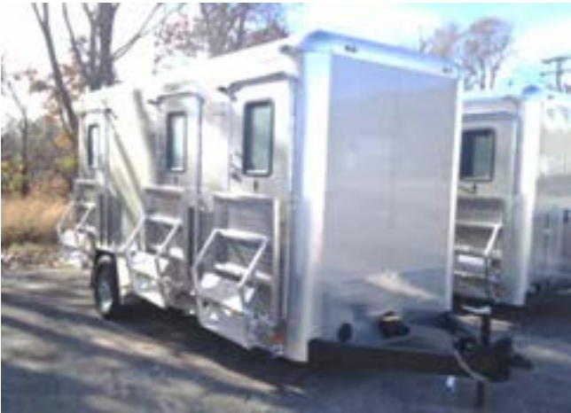
View of the Trailer with Steps and Porches Retracted. Railings are Stored in the Front Carrier
