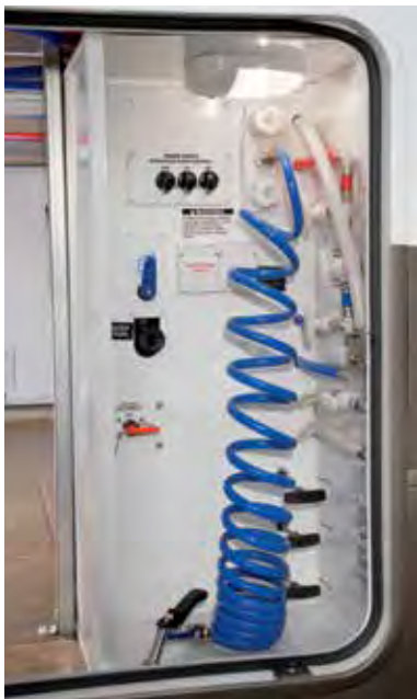
The Docking Station includes outside shower, black tank flush, water bypass, 12V battery disconnect, selector switches, dump valves, water tank and city fills for centralized convenience.
