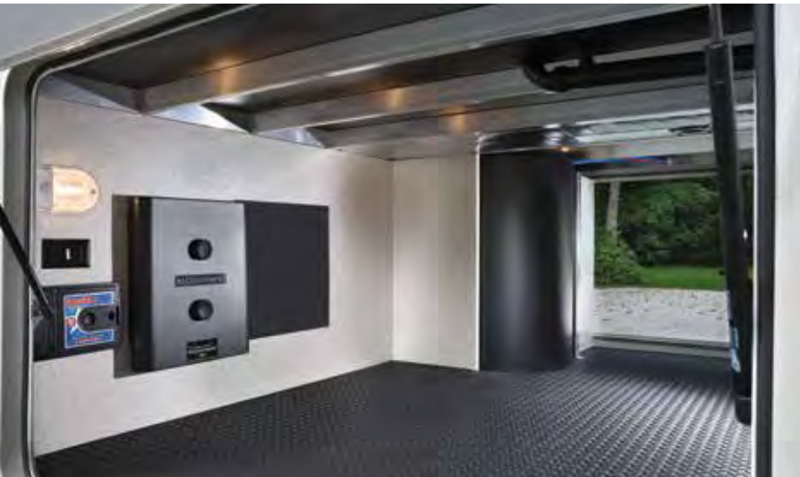
Hathaway's Z-frame, heated front storage compartment provides over 100 cu. ft. of storage and includes an extra vacuum port for outside clean-ups.
