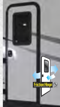
Main Entry Door with Friction Hinge
