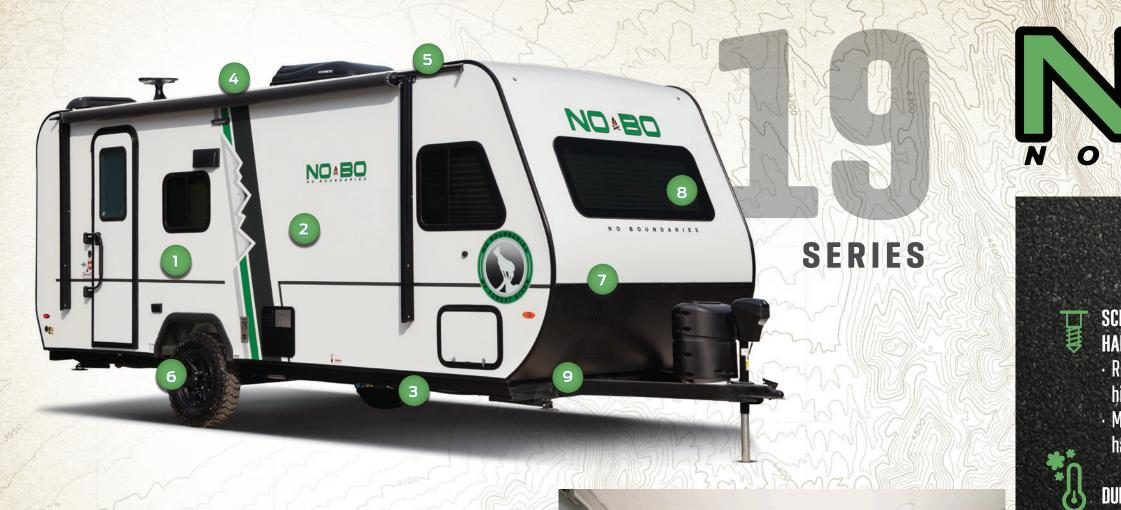
**Aluminum Construction and** Laminated Side Walls - Welded aluminum framing around all opening resulting in the best structural integrity in its class. Pinch roll laminated AZDEL construction with 100% glue coverage.
