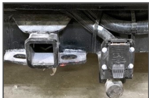
BRAKE SYNC Brake Sync Tow System pre-installed from Freightliner for quick connect for tow vehicle air braking system.
