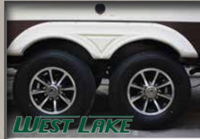
Contemporary aluminum rims with E-rated radial tires. All SIERRA's feature 7000 Lb. axles.
