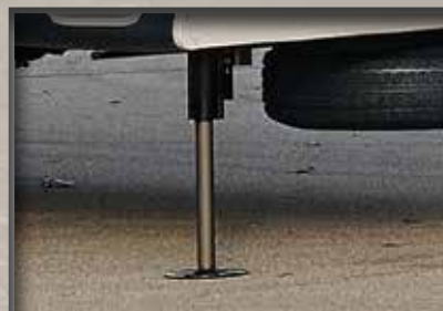
Wide stance power front jacks. (Optional hydraulic jacks shown, 14 times faster than electric jacks.)
