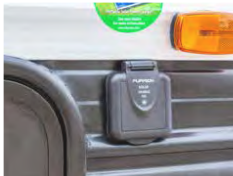
Solar Prep and Wiring
