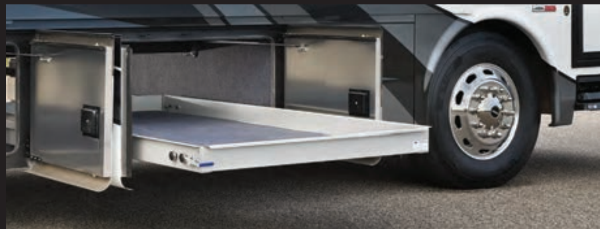
STANDARD SLIDE TRAY IN STEEL BASEMENT FULL PASS THRU STORAGE COMPARTMENT
