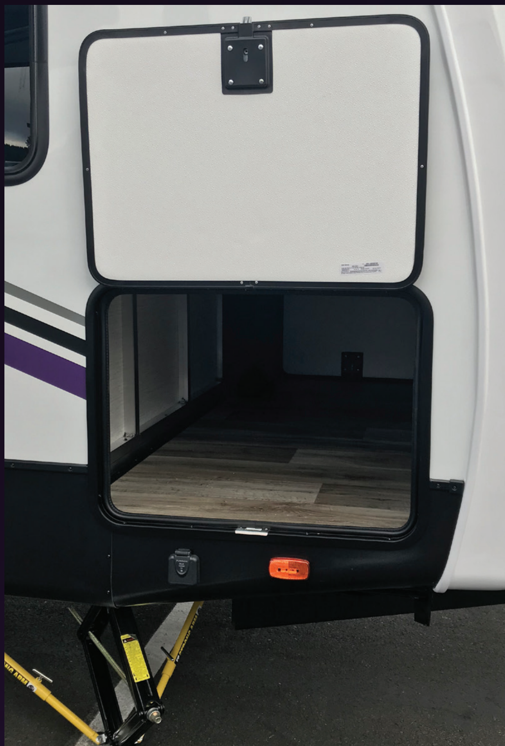
Oversized 32" x 24" Slam Latch, 1" Insulated Baggage Doors (Large enough for a standard Generator) JT Strong Arm™ Stabilizer System Magnetic Door Catches
