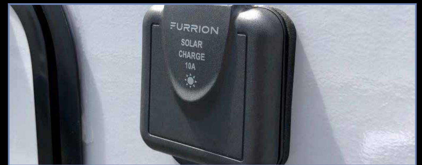
Side Solar Prep and Wiring
