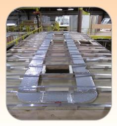
Our 5" aluminum roof rafters allow us to run a full 8" wide, race track, duct system. This allows more ducted air flow compared to our competitors 5" wide duct. Circular ducting ensures uniform cooling with (1) standard air conditioner or upgrading to an optional 2 air conditioning system.
