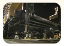
jacks are tested right on the production line to ensure proper working order. This process eliminates air bubbles within the hydraulic lines.
