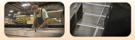
Cedar Creek's walls sit <u>on top</u> of the floor and are bolted to the outrigger. This allows for full aluminum framing around all windows and doors.
