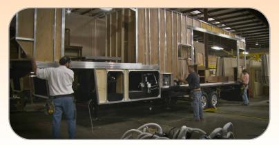
**Individually fastened, custom "L" brackets** are combined with Silaprene adhesives that are designed to bend, flex and absorb road stress. Silaprene adhesives have a 475 PSI *(Pounds per Square Inch)* and get stronger as it ages. It is resilient and has outstanding resistance to moisture, road chemicals, heat, and cold.
