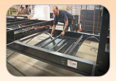
Inserted into each steel frame is our one of a kind, ABS, impact resistant, waterproof, underbelly. Each 4' x 6' ABS panel is inserted front to back, inside each frame. The panels are then anchored into a braced wood backer within the frame.
