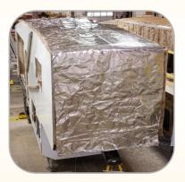
Triple layered residential insulation is installed including a Radiant Thermo-Foil, with an R-value of 38, which is wrapped underneath the front cap.
