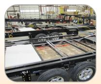
Black, Grey, and Fresh Water tanks are installed with individual 12-volt, large surface heating pads on *ALL* tanks. These tank heaters allow for all season camping.
