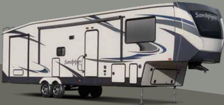
GVWR (Gross Vehicle Weight Rating) - is the maximum permissible weight of the unit when fully loaded. It includes all weights, inclusive of all fluids, cargo, optional equipment and accessories. For safety and product performance do NOT exceed the GVWR.
