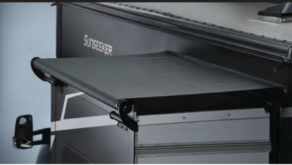
Slide out awning toppers help keep water and debris off the top of your slide rooms
