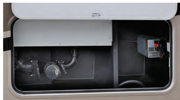
Heated/enclosed holding tanks use warm air from the furnace to protect tanks and valves. (N/A on 2250DSLE and 2550DSLE)
