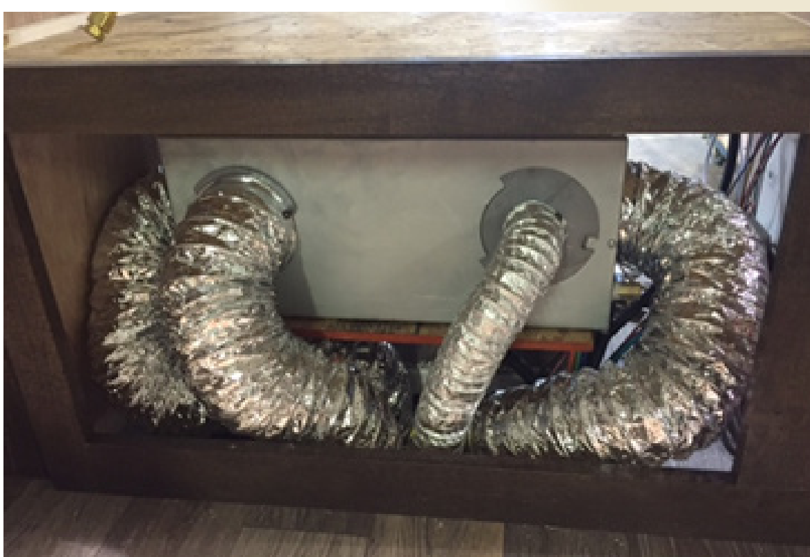
Enclosed & heated underbelly w/2" forced air heat into enclosure; optional 12V heat pads
