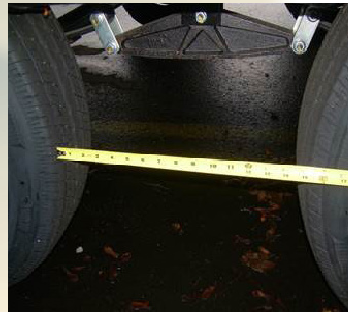
Wide-track spaced axles provide better stability and handling while towing
