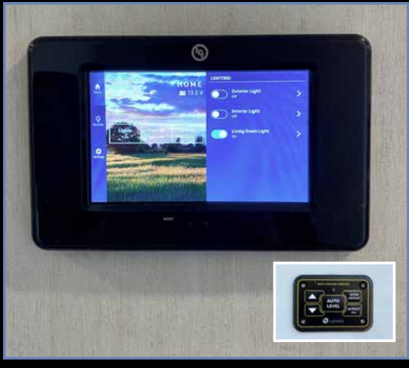
Automatic Leveling and Stabilization System with Hitch Memory and Dual Control Accessibility
