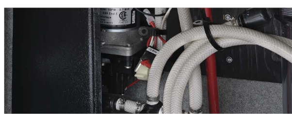
Winterizing tube provides easy access for quick maintenance; includes bypass valve (N/A 2251SLE, 2551DSLE)
