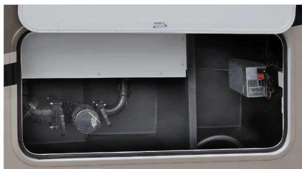
Heated/enclosed holding tanks use warm air from the furnace to protect tanks and valves (N/A on 2251DSLE and 2551DSLE)
